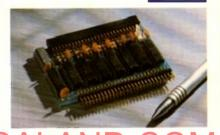
Expand your A500's memory up to a total of 2MB without disposing of your existing 512K upgrade (works with 1MB chip RAM, 512K RAM must be 4 chip type or not exceeding 9cm in length. Your Amiga needs to be opened, this may effect your warranty).
