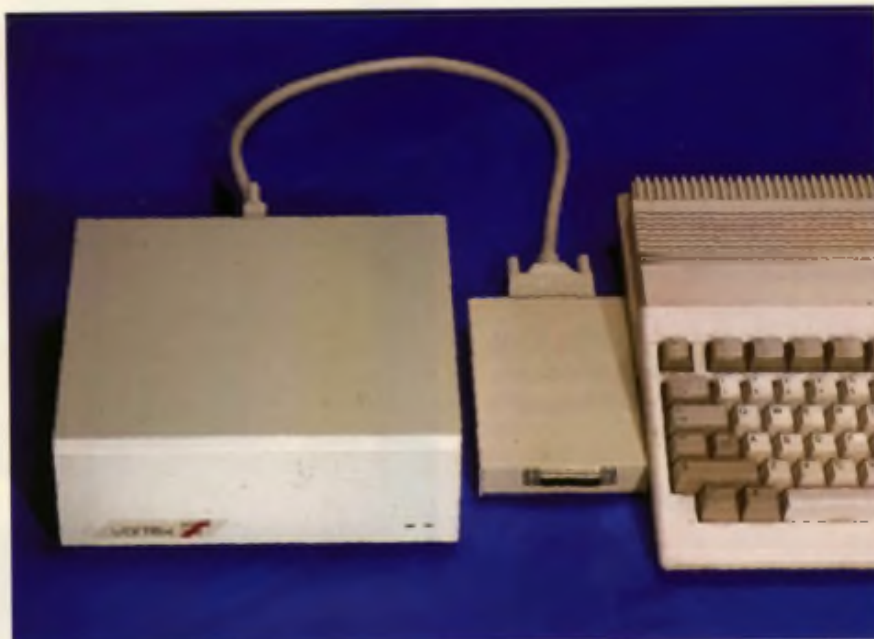
Vortex's System 2000 is connected to the Amiga via a device called the personality module which is included with the system. Unfortunately, the HD offers no expansion ports except an extra drive port and isn't particularly fast. Phantom errors are also another problem.
